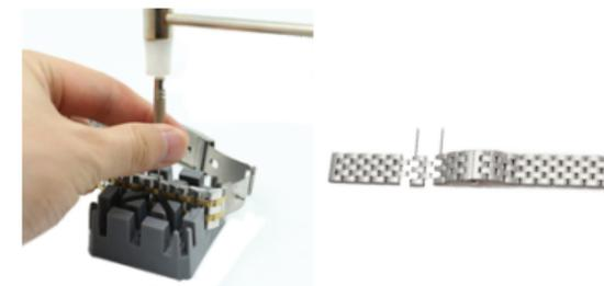
Step 1. Use something to hold the band, push the adjust needle into chain hole, pull out the spring bar.
